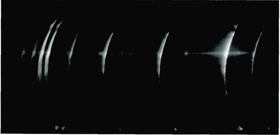
Fig. 8. Flash spectrum of the chromosphere obtained with a pair of objective prisms and a 2x conversion lens attached to an 8 cm refractor. Strong emission lines visible on the spectrogram are, from right to left,  $H\alpha$   $\lambda 6563$ ,  $HeI D_3$   $\lambda 5876$ ,  $H\beta$   $\lambda 4861$ ,  $H\gamma$   $\lambda 4341$ ,  $CaII H$   $\lambda 3968$  and  $CaII K$   $\lambda 3934$ , respectively. The splitting of the line is due to miss-alignment of the two prisms.
