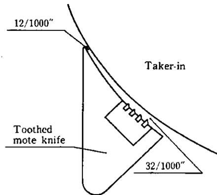
**Fig. 2** Settings between the toothed mote knife and the taker-in roller
