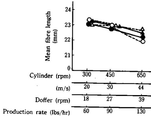
Fig. 7 Mean fibre length of sliver (with Fibrograph)
